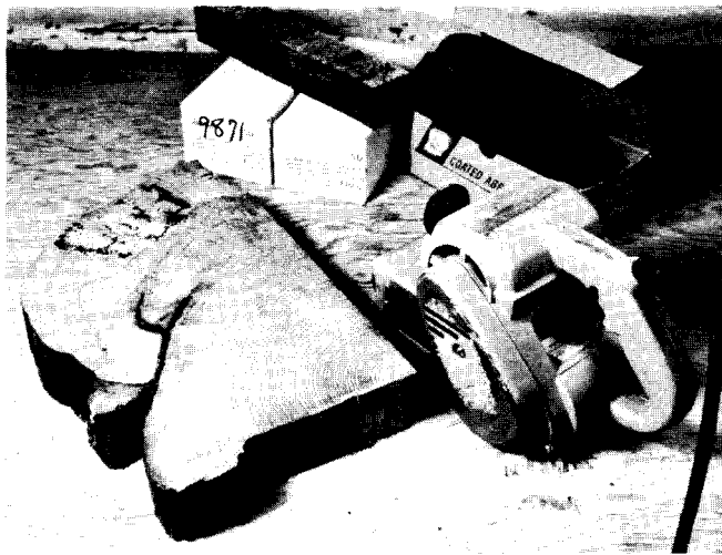
Figure 7 —Belt sander and gum-cleaning bar for preparing surface of cross sections.
