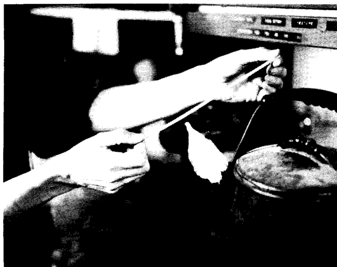
Figure 5 —Straightening a twisted core over a jet of steam.
