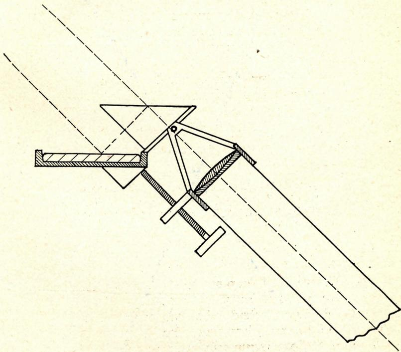
It is not difficult to understand that this device accomplishes this result. When the two images of any star are in coincidence, the reflecting surface of the prism must be parallel to the surface of the mercury and therefore perfectly horizontal. Hence at any azimuth the coincidence of the stellar images indicates that the reflecting surface of the prism is perfectly horizontal and therefore that the telescope is pointing at the zenith distance for which the instrument is adjusted.
